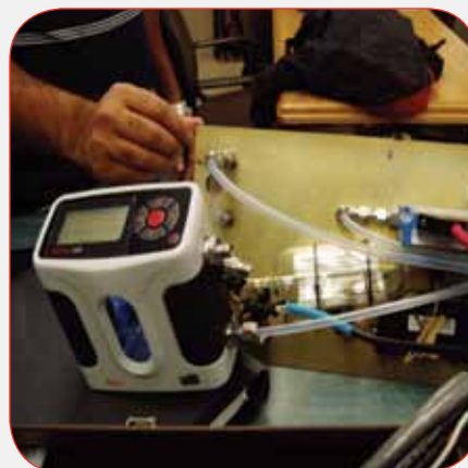
Fig 2: Bios DryCal connected to gas dilution calibrator
