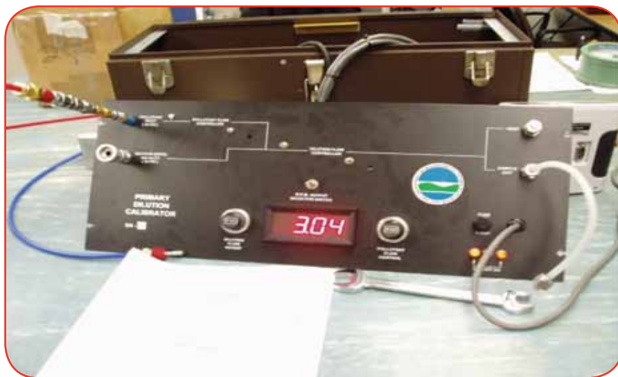
Fig 1: EPA Primary Gas Dilution Calibrator
