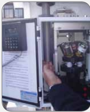
Figure 2: Raising the down tube
