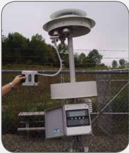
Figure 1: Bios Definer™ 220 Connected to SuperSASS Sampler
