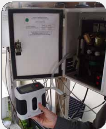
Figure 1: Bios Definer 220 connected to IMPROVE Sampler
